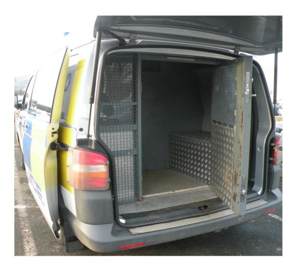
3.17 The cell door mechanism was designed so that when the door is closed the spring loaded latch bolts would retract and then fall/lock into the relevant recess in the floor. When this was done the door cannot be opened without turning the door handle at the rear. It was established that if the latch bolts did not engage then the door can be opened with little or no pressure and without using the door handle.
