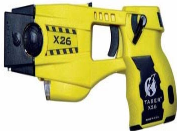
The X26 model of Taser has an audit functionality which records the date, time, temperature, battery condition and duration for which the Taser was discharged. Each Taser has a memory of 1500 incidents, and the information recorded for each is downloadable for police and Police Ombudsman records.
